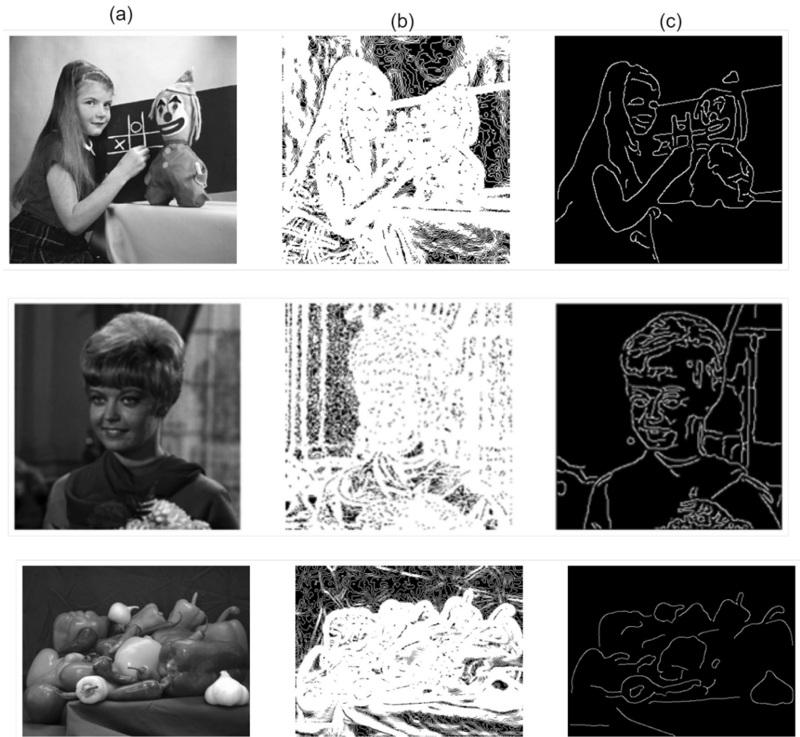
Fig. 21. (a) Original image, (b) image after applying QED of AFQIRHSI, and (c) Canny edge detection method.
