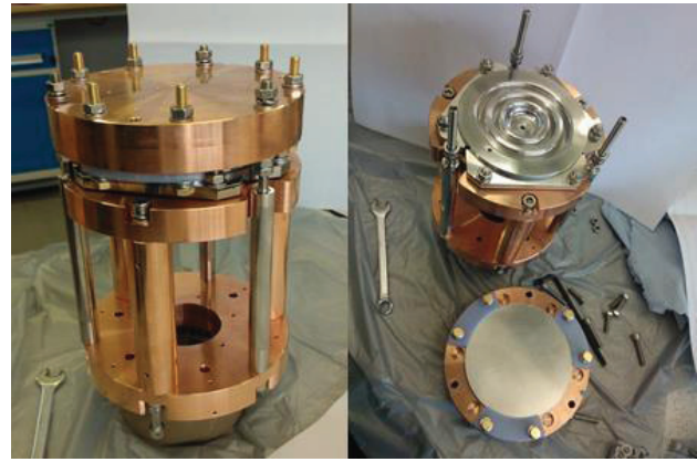
Figure 6: Test assembly of the cavity and sample mounted in its support cradle.
