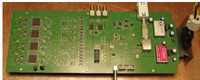
Figure 4: Test-board for the NECTAr0 chip. Four NECTAr0 chip are soldered on the top of the board (on the left) and four more are soldered under the board.
