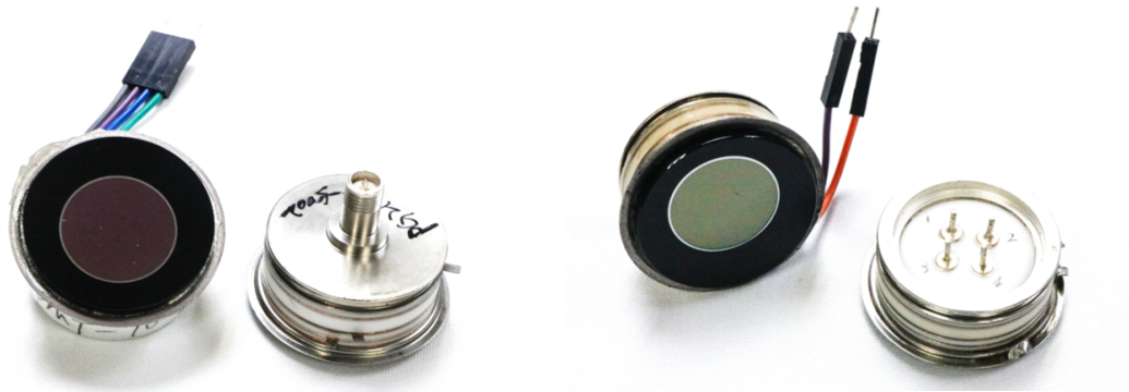
Figure 4. Round single-anode FPMT prototype. Figure 5. Round 2×2 anode FPMT prototype.
