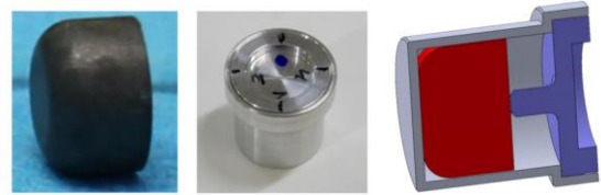
Fig. 1. From left to right: ^{238}\text{U} sample before and after encapsulation, scheme of the encapsulation (red: sample, grey: aluminum container, blue: aluminum plug).
