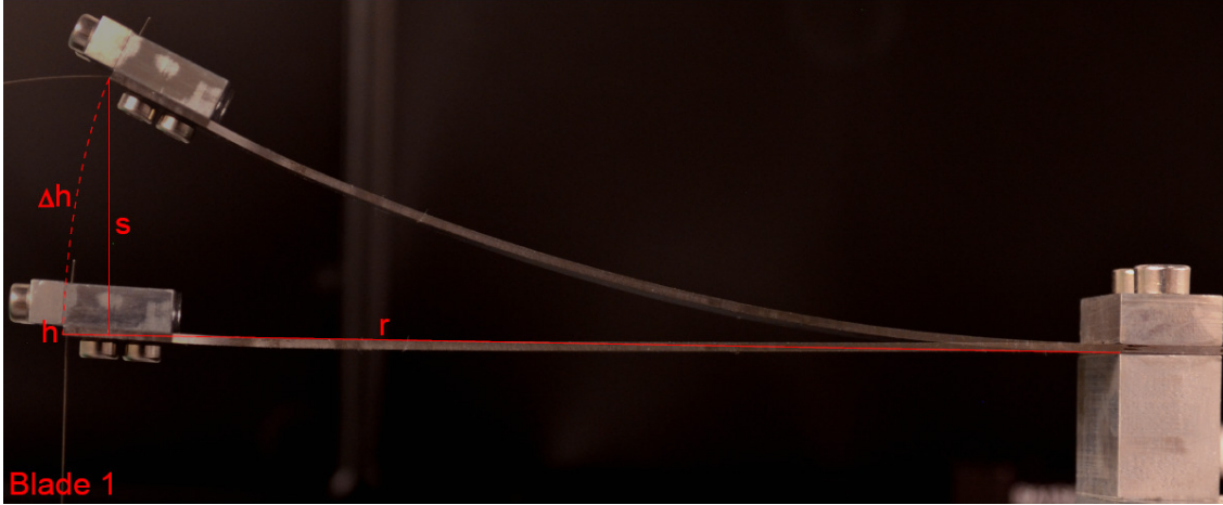
Figure A.2: Here, the BS suspension's blade spring characterization using a camera picture can be seen. Parameter values for the different blade springs are shown in table A.1
