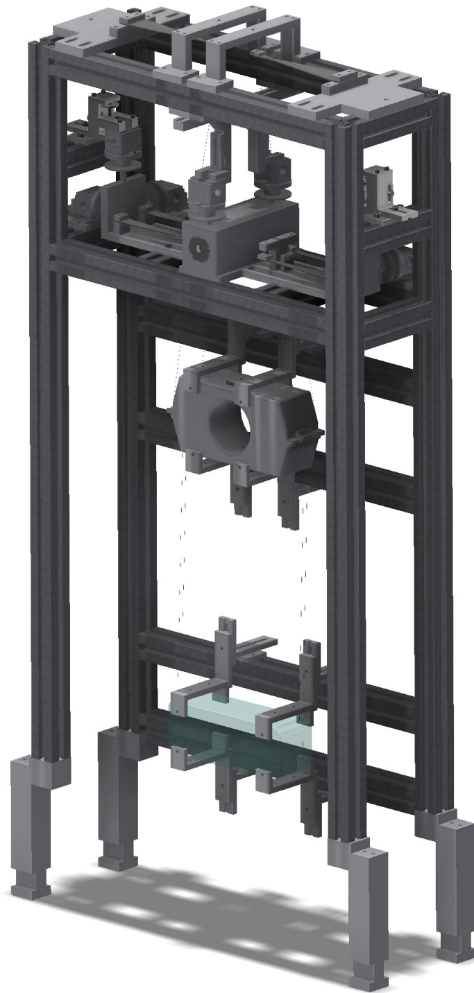
Figure 4.14: CAD picture of BS triple suspension. Suspension cage made from 30 mm x 30 mm aluminum profiles. The top carries two blade springs, forming the first vertical suspension stage. The BOSEMs are attached to the suspension cage, measuring and actuating the motion of the first suspension stage.
