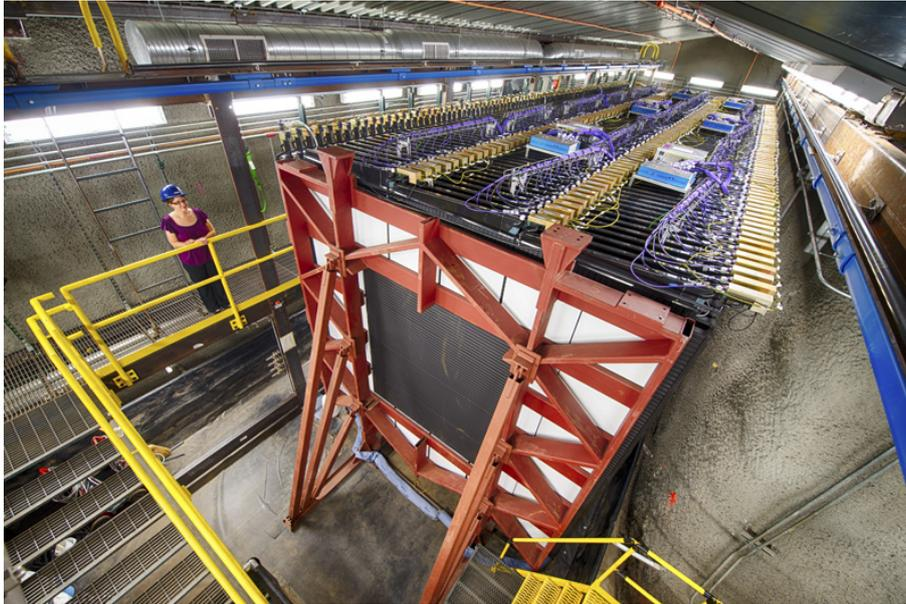
Figure 3.9: The NOvA Near Detector located at Fermilab. The ND is housed underground and 1 km away from the NuMI beamline. From [38].
