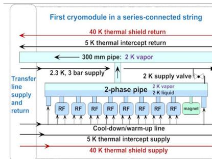
Figure 2: Cryogenic flow schematic of a 1.3 GHz LCLS-II cryomodule.
