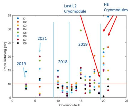
Figure 3: Cavity peak detuning of all 8 cavities from cavities tested from 2018 until 2022. These include cavities from LCLS-II and HE. The cavity peak detuning specification is 10 Hz.
