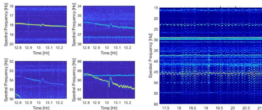
Figure 6: Spectrograms showing harmonics observed in cavity 7 in CM 15, the fundamental mode occurs at rightly 18 Hz and the higher order modes are shown.
