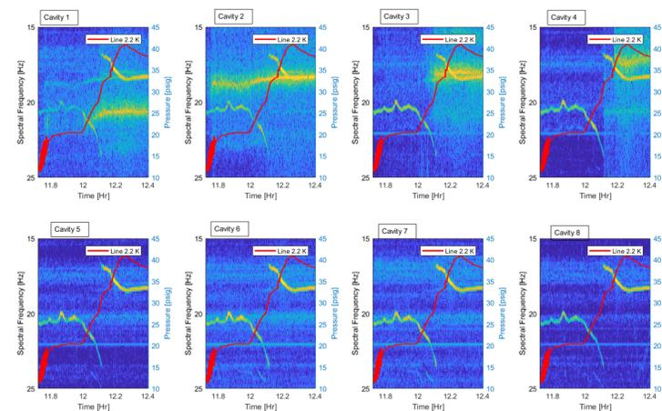
Figure 5: Spectrogram of the cavities in vCM showing the transition of 20 Hz vibration to 18 Hz by changing the supply pressure of the 2.3 K line.
