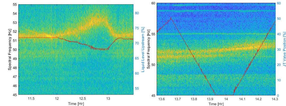
Figure 8: Liquid level variation for Helmholtz mode in cavity 1 CM21. The liquid level is correlated with the 51.5 Hz mode.
