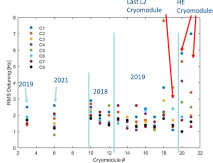
Figure 4: RMS cavity detuning from 2018 to 2022. These include cavities from LCLS-II and HE.
