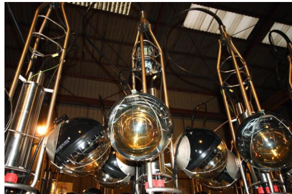
Figure 1. An image of ANTARES OMs mounted on 3 storeys. The large PMTs are visible inside the glass spheres. The LCMs (the cylinders) are also visible.
