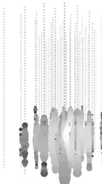
Figure 5: Cascade event in IceCube-40. Small dots are position of DOMs, circles show light received, where size indicates number of photons.
