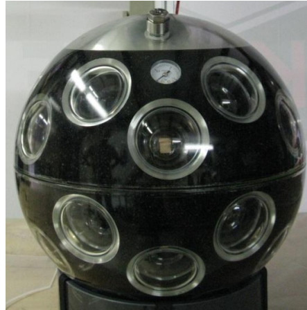
Figure 1: The KM3NeT DOM showing the photomultipliers with the light concentrator rings, the foam support, the aluminium cooling structure and the blanked cable feed-through.
