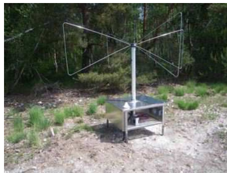
Figure 4: Picture of a standalone detector being deployed on the field.
