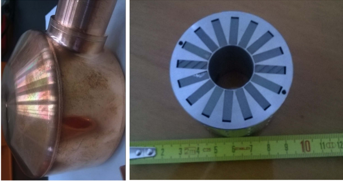
Figure 29. Drift tube linac component prototypes (Courtesy of INFN-LNL). Left: a drift tube body. Right: a permanent magnet quadrupole that is inserted inside the drift tube body.
