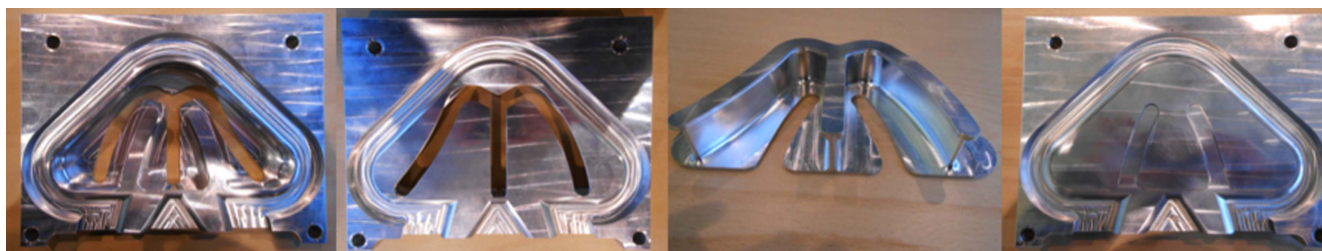
Figure 84. Cold moderator halves milled from two solid AL6061-T6 work pieces. From left to right: lower half; lower half turned; upper half; lower and upper halves together [142].
