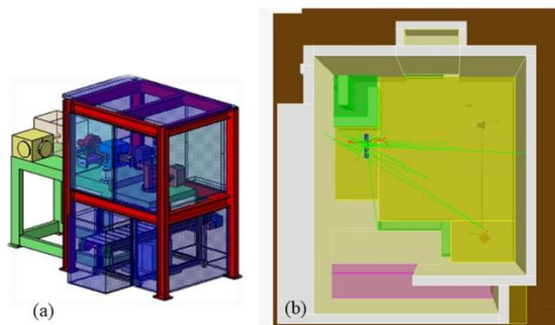
Figure 3: Two scenarios for radiation shielding: (a) extra steel shielding box and (b) layout of steel plate covering the accelerator hall.
