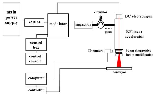
Figure 1: Diagram of the RF-linac system for natural rubber vulcanization at Chiang Mai University.
