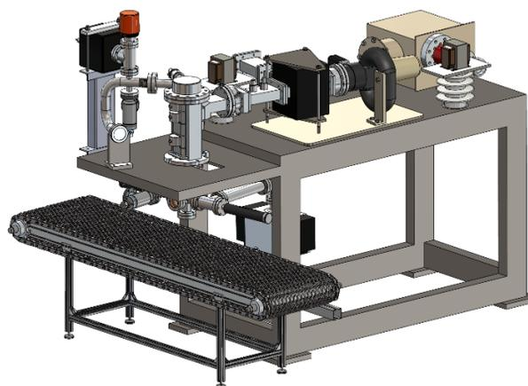
Figure 2: Layout of the accelerator system consisting of a DC-gun, a linac, a magnetron and a conveyor under the beamline.
