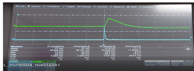
Figure 6: Bench test result of BPM active filter using 2SC4083.
