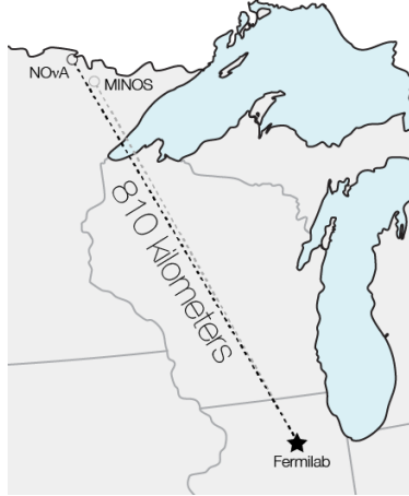
Figure 3.4: The NOvA baseline. Geography both political and physical has enormous impacts on experiment design considerations for these large experiments.
