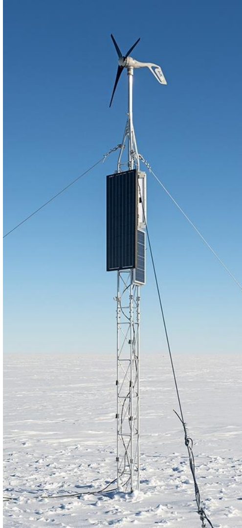
Figure 1-1: An ARIANNA station on the ice. Photo by Dr. Stuart Kleinfelder.
