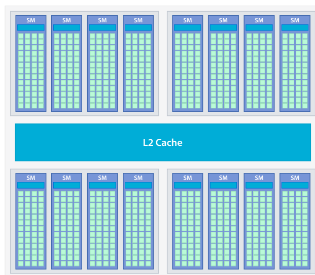
Figure 4.2: Sketch of the multiprocessor and memory distribution on a GPU. Cache is colored in blue, a Streaming Multiprocessor is colored in purple, with the individual cores sketched in green.
