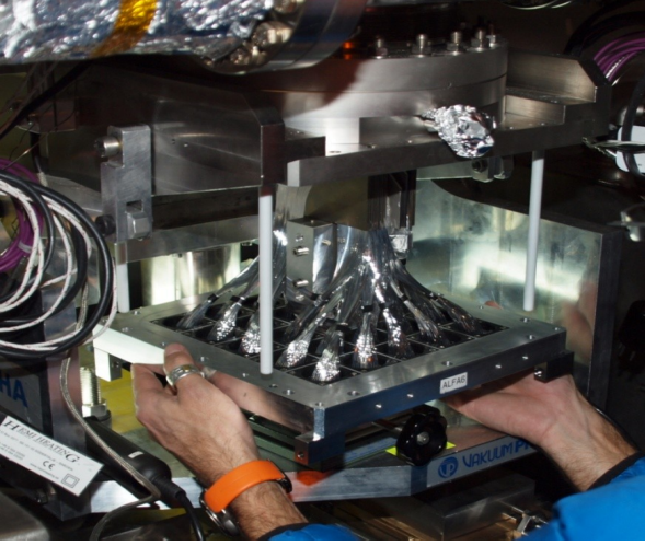
Fig.5: Insertion of a lower fibre detector in the RomanPot.
