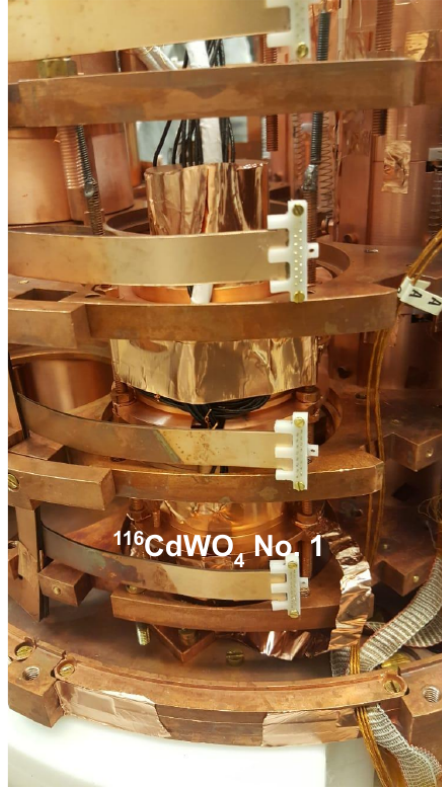
FIGURE 5.5: The ^{116}\text{CdWO}_4 scintillating bolometer installed in the EDELWEISS cryostat.
