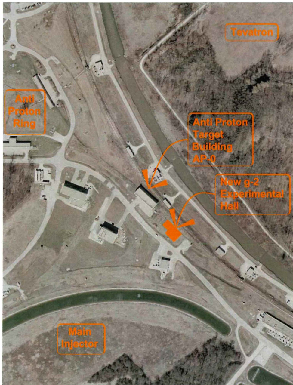
Figure 3 – g-2 Experimental Hall Site Plan
