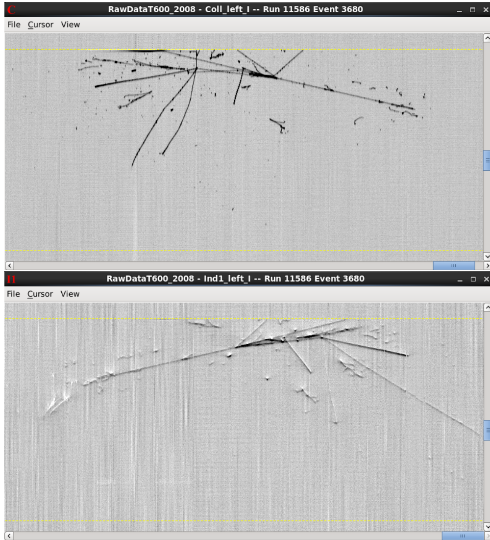
Figure 8.2: Run 11586 Event 3680 is classified as vertex event(3 classification). There is again the PMT interference seen in the collection view (coll window). This event might have been the result of a nuclear interaction.
