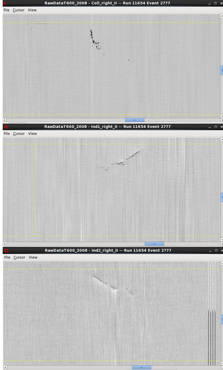
Figure 10.4: This iBDM candidate(Run 11654 event 2777) upon closer inspection only contains one part of the iBDM topology ( e^+e^- ). This event could have been produced by a stray gamma ray. For this reason, the event was rejected.
