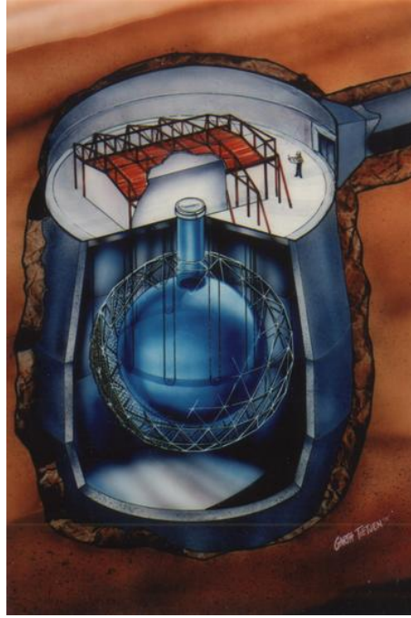
Figure 1.3: An artist's illustration of the SNO detector.
