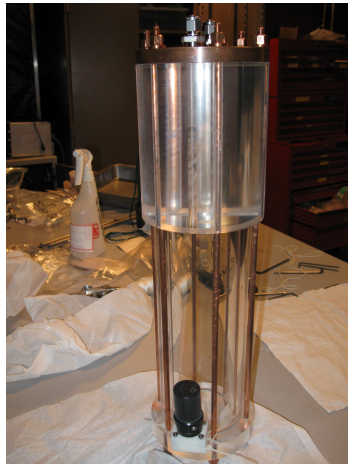
Figure 3.1: A photo of the scintillator bucket with the AmBe neutron source (black cylinder) beside it.
