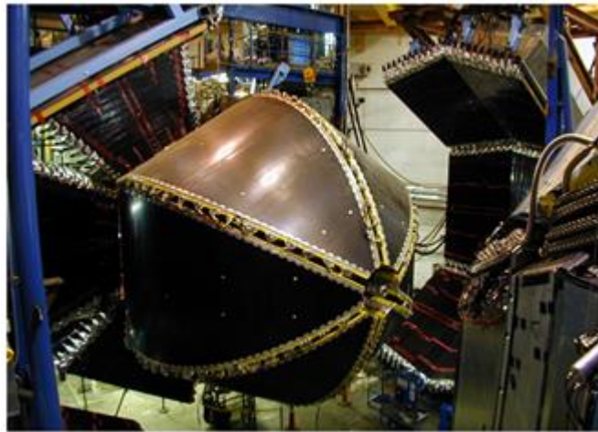
Fig. 1. The CLAS detector in an open maintenance position exposing the large drift chambers covering nearly the full polar angle range. The time-of-flight scintillator bars and the forward electromagnetic calorimeters are also visible.
