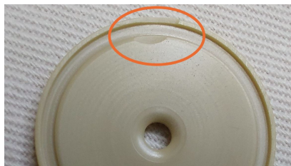
Figure 3: Example of damaged ceramic that could not be used for assembly.
