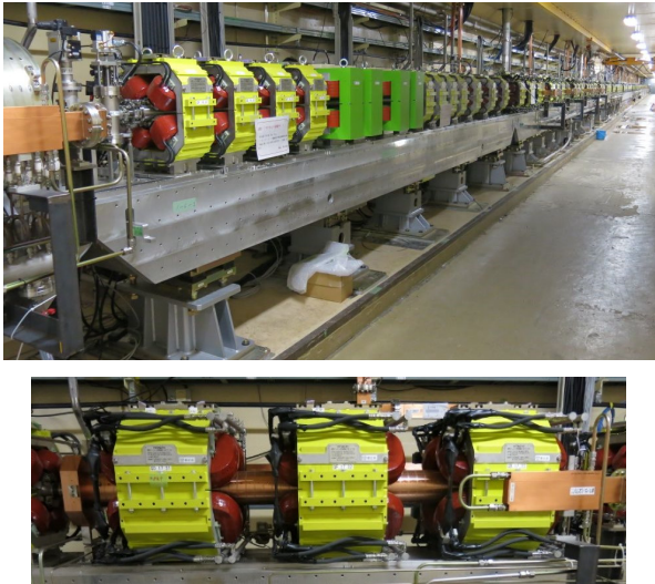
Figure 6: Densely placed quadrupole magnets for transportation of large emittance positrons. They are overlapping with the accelerating structures.
