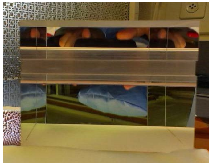
Fig. 5.4: View of focusing block after covering the cylindrical surface with an aluminum coating. Viewing angle is into the focusing block, showing the mirrored cylindrical focusing surface.
