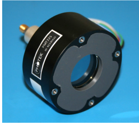
Fig. 3.3: Frontal view of a TORCH Phase 1 MCP-PMT [50].
