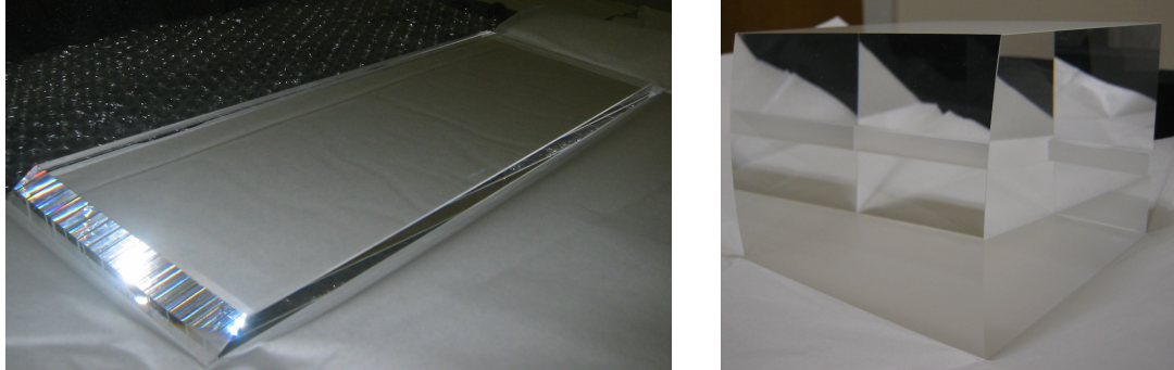
Fig. 5.3: Quartz acquired from Schott for the TORCH testbeam prototype. (Left) The radiator plate of size 120 \times 350 mm with a bevel on the top, of which the sharp angle is 36^\circ . (Right) Matching focusing block of width 120 mm, with a cylindrical surface with focal distance 260 mm, matching the design shown in Figure 4.3.
