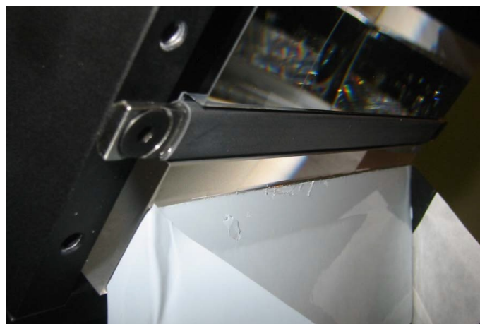
Fig. 5.7: TORCH optical assembly after gluing the radiator and the focusing block together with a 50 \mu\text{m} thick layer of Pactan 8030. The radiator is covered with a layer of plastic for protection.
