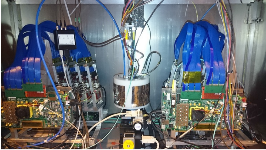
Fig. 5.10: VELO Timepix3 telescope, situated at the SPS testbeam facility at CERN [109].
