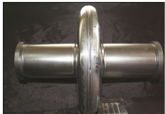
Fig. 6. EB welded Cavity (after final welding)
