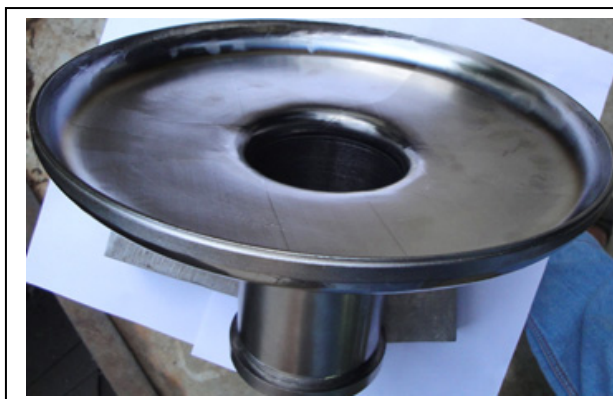
Fig.5. Half cell to beam tube assembly
