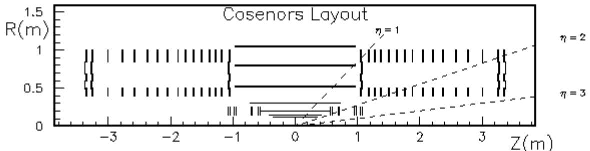
Each detector consists of line ‘elements’ which represent silicon crystals folded through  $2\pi$  in the barrel, or MSGC/GaAs rings in the end-cap. Conceptually, each detector element corresponds to a row in the ‘geometry table’. The lines are replaced by thin rectangles to take into account factors such as the tilt angle of the barrel detector for tiling and Lorenz angle compensation, as shown by zooming in onto part of the SIT detector:
