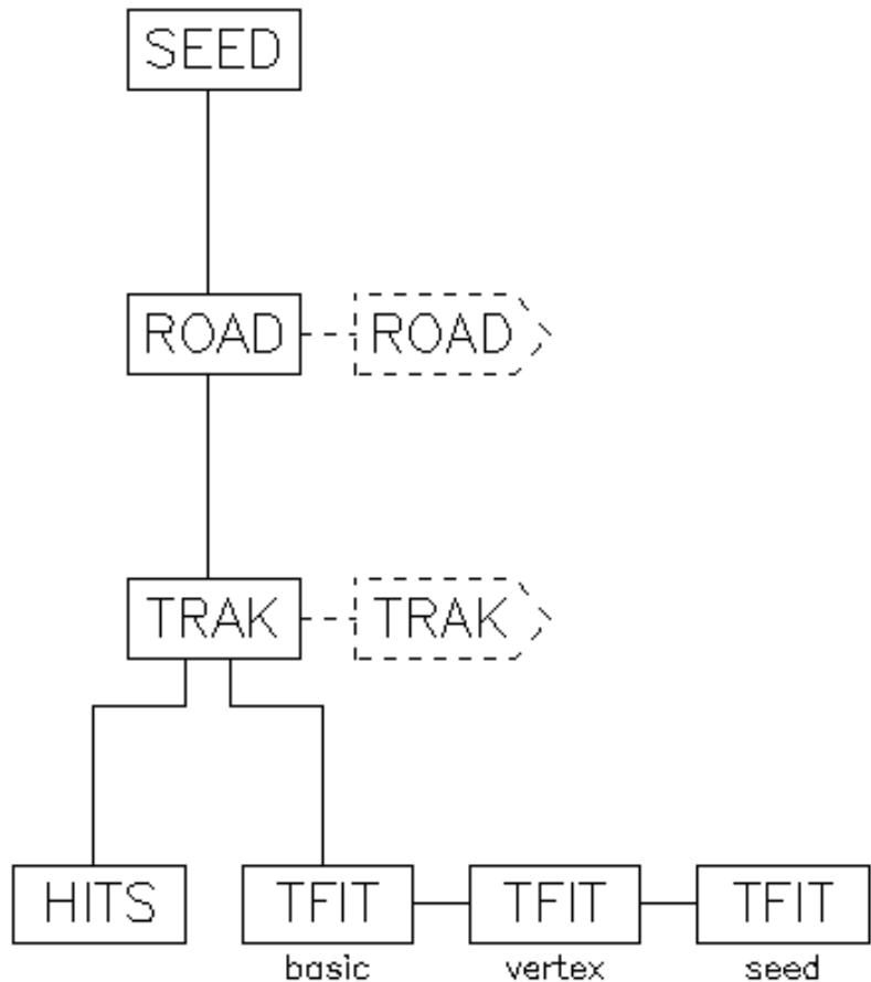
Details of each ‘trigger’ seed considered, along with its corresponding vertex region, transverse momenta and  $\chi^2$  cut-offs, are to be found in a horizontal chain of ‘ROAD’ banks. In turn each ‘ROAD’ supports a horizontal chain of ‘TRAK’ banks, one for each track found in the road. Each successful track has 3 types of track-fit stored in ‘TFIT’ banks and the associated tracking detector hits stored in the ‘HITS’ bank. There is a ‘basic’ fit to the asso-
