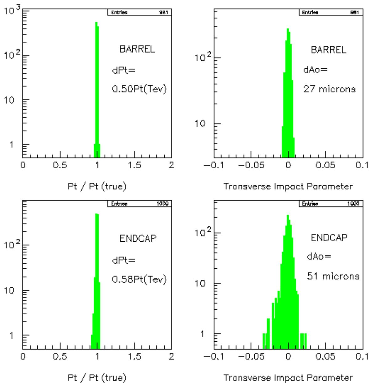
Muon triggers (seeds) were created as electromagnetic clusters by enhancing the energy deposition of the muons in the calorimeter. To test the correctness of the program 20GeV muons were generated with all physics processes turned off. The barrel and end-cap performances are contrasted in the preceding figure. It is seen that the barrel is more precise than the end-caps for impact parameter physics, whereas barrel and end-caps are reasonably well balanced for momentum resolution measurement.
