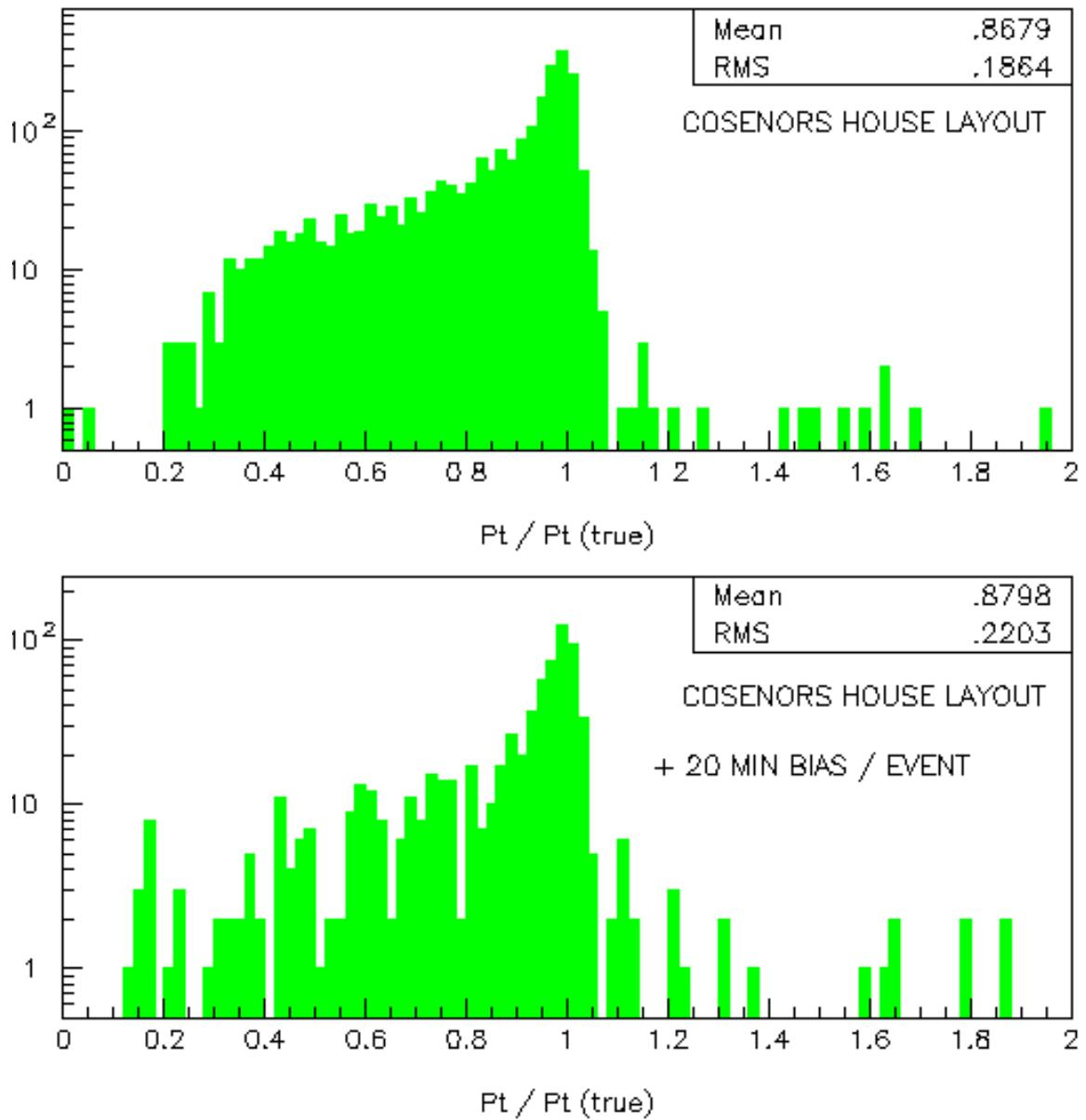
All runs made with muons, give a track finding inefficiency per trigger of ~1%, dominantly caused by the alignment of the MSGC frames in  $\phi$ . For electrons the inefficiencies are of the order of 5% at 20 GeV due to bremsstrahlung. This will be reduced when the special electron fit is introduced.
