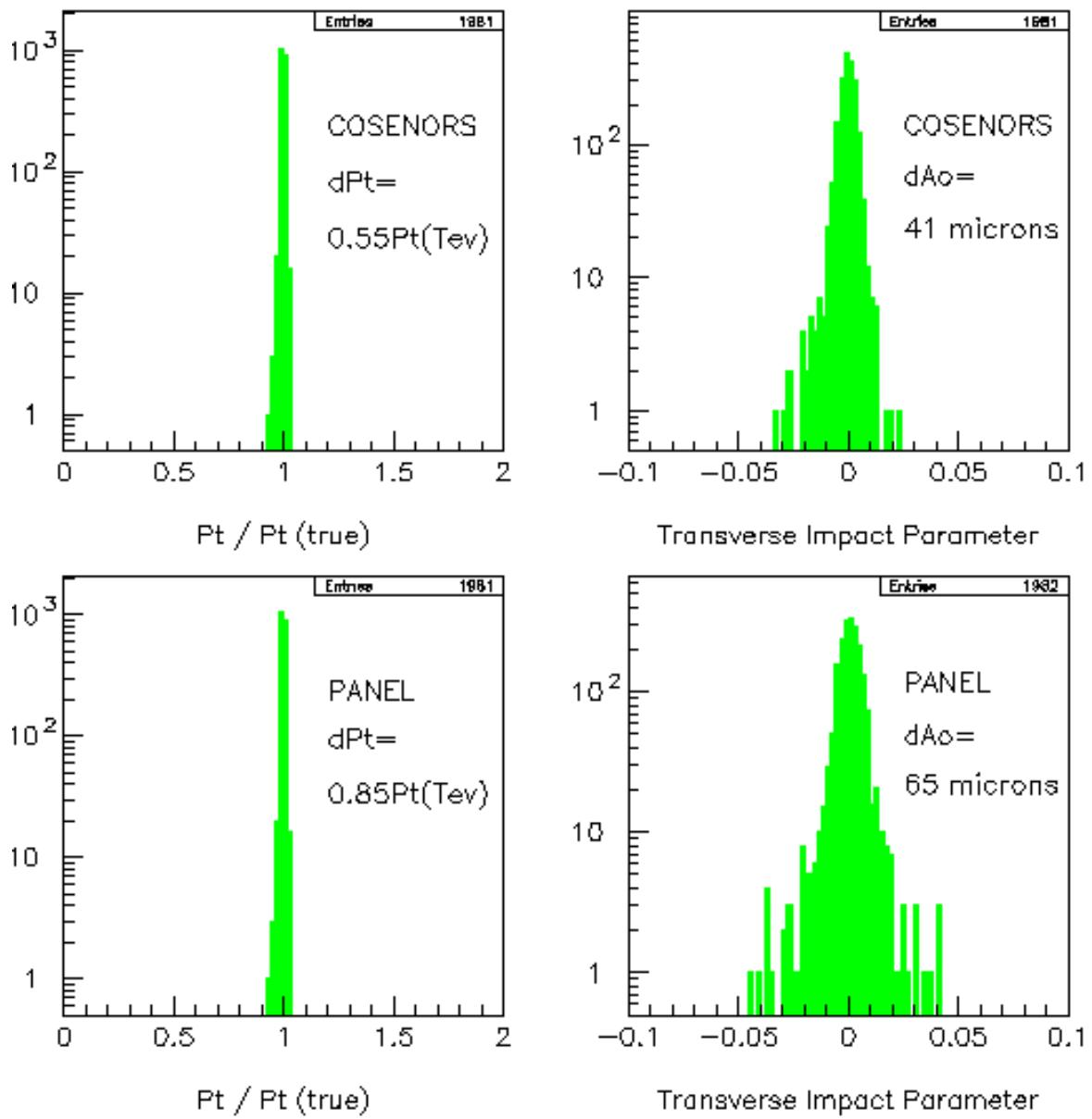
Minimum values for  $\Delta p_T/p_T$  of  $0.55 p_T$  (Tev), and  $0.85 p_T$  (Tev), are found for the Cosenors House and Panel layouts respectively. Of course the addition of precision TRT measurements should reduce this difference.
