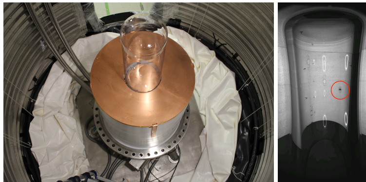
Figure 3. Left side: View from the top showing the assembled inner vessel section of the PICO-40L experiment. Right side: one of the first bubbles recorded with PICO-40L, bubble highlighted by a red circle.
