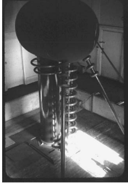
Fig. 7.1. The insulating column on the Melbourne University Van de Graaff has two corona rings near the terminal. These reduce the electric stress on the column adjacent to the terminal by spreading portions of it to the regions at the corona rings
