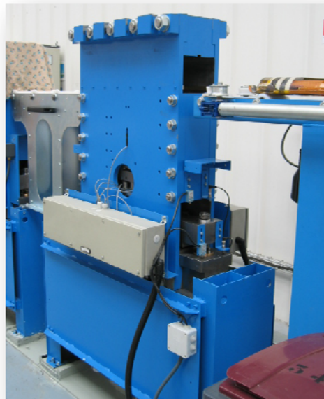
Figure A.17 _ Device for Young’s modulus measurements at Jeumont.
