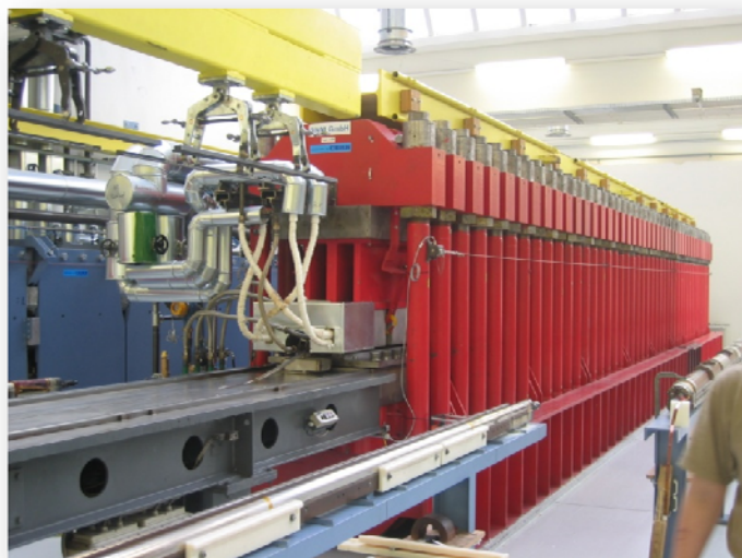
Figure A.8 _ Curing press at Noell.
