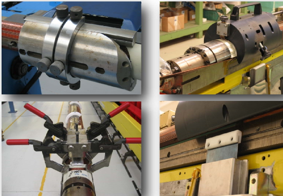
Figure A.12 _ Some of the fixtures used by the MP's to support cables during winding: at Jeumont (top-left corner), at Ansaldo (right column) and at Noel (bottom-left corner).
