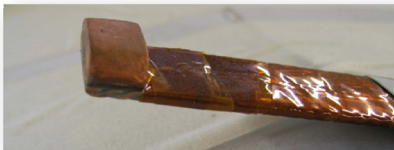
Figure A.10 _ Cu block soldered on outer layer cable extremity at Ansaldo.
