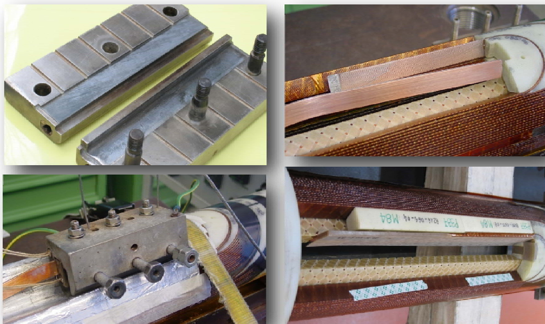
Figure A.18 _ Left column: on the top, splicing tooling at Jeumont; on the bottom, tooling at Ansaldo. Right column: splice before and after formation.
