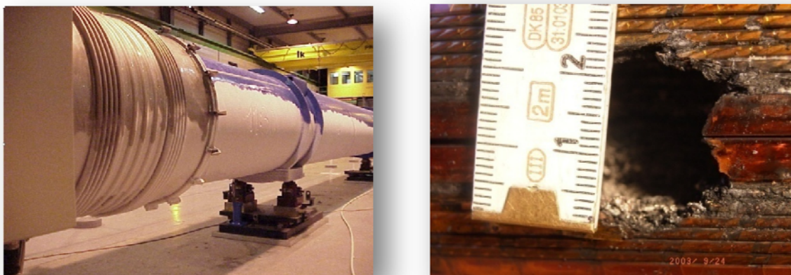
Figure 3.3 _ Effect of an electrical short.
