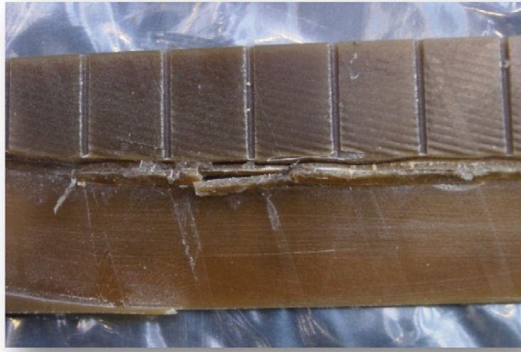
Figure 3.15 _ Fracture of G10 support for the layer jump.
