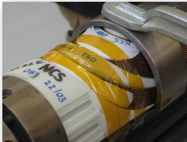
Figure A.13 _ Example of Teflon fillers added at Noell on conductor blocks.
