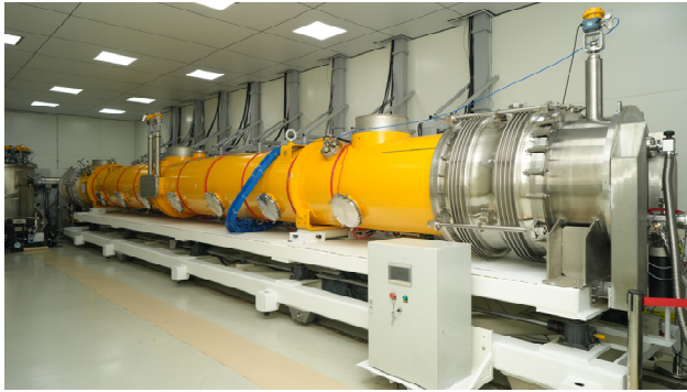
Figure 1: 1.3 GHz cryomodule with eight mid-T bake 9-cell cavities in the horizontal test stand at IHEP's Platform of Advanced Photon Source (PAPS), Huairou, Beijing.
