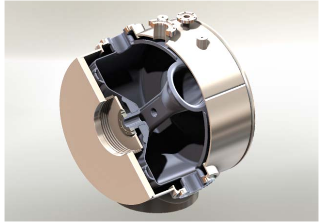
Figure 6: Sectioned view of the SSR1 resonator inside its helium vessel. The different materials are shown with different colors.
