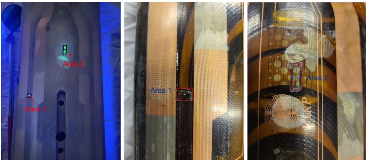
Figure 6.5: Areas where dye emerged on coil 214 outer surface in the Lead End
