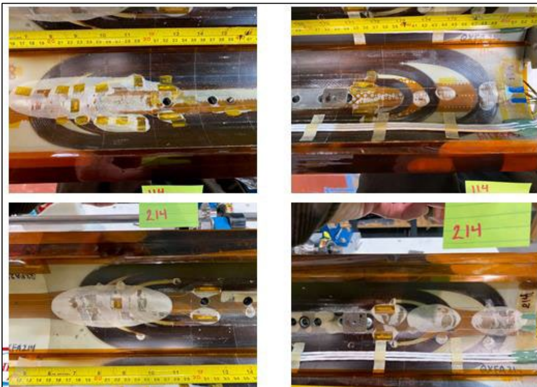
Figure 4.7: Inner surface of coil 114 and 214 in the end region after test.
