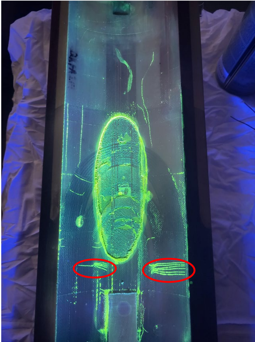
Figure 6.6: Inner surface of the Lead End showing some cracks on the surface of the epoxy-impregnated insulation layer. After the go-through inspection, the dye penetrant was cleaned on the inner surface and revelator was applied on the same surface to get this picture. The red ovals show the marks located/starting at the interface between wedges and end-spacers.
