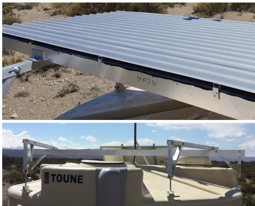
Figure 6. Top: the sunroof of the SSD consisting of corrugated aluminium sheets. Bottom: the SSD support structure on top of a WCD tank.
