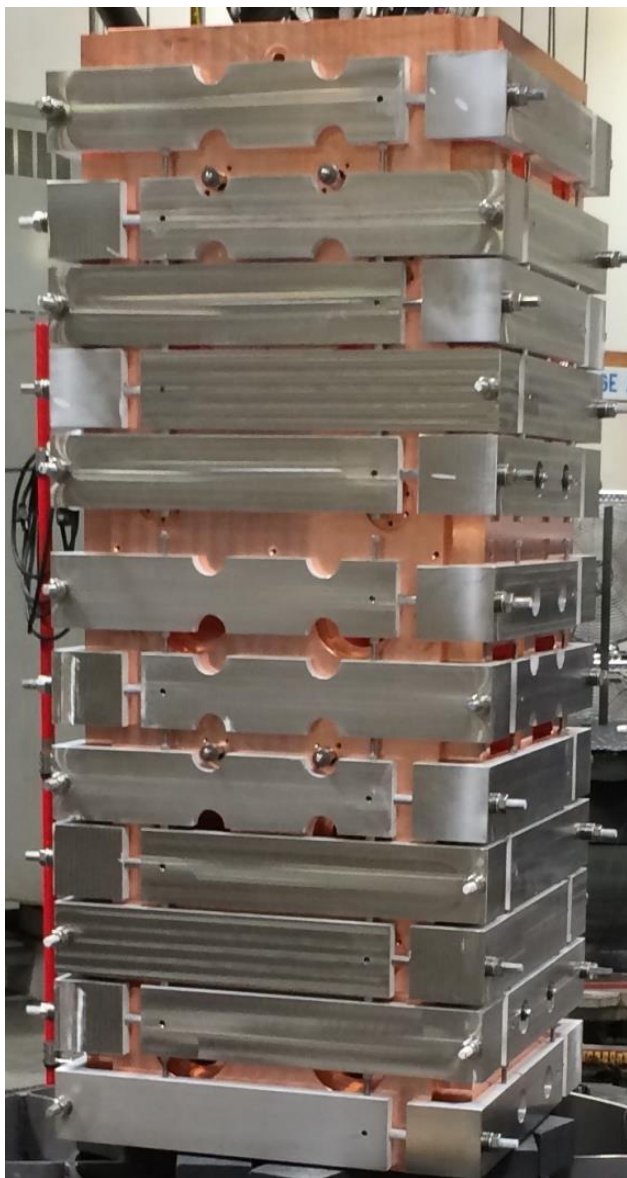
Figure 6: RFQ module with braze fixtures.
