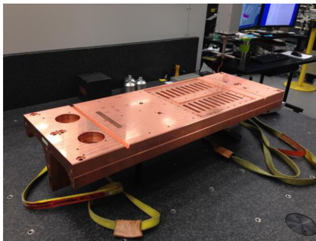
Figure 1: Backside port CMM check.
