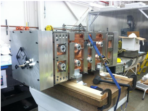
Figure 4: LBNL module 2 prep for bead pull.
