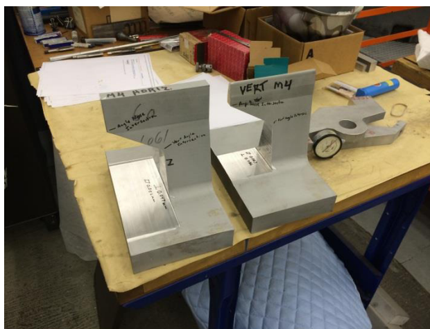
Figure 2: Aluminum test pieces to verify cutback machining program, if acceptable the program is saved on machine to be duplicated on the production part.
