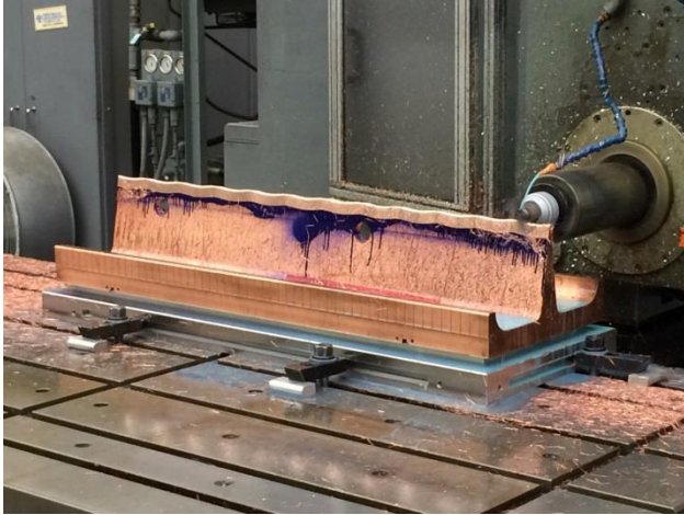
Figure 3: Vane modulations being cut at LBNL
