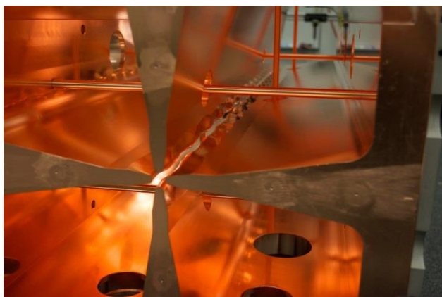
Figure 7: Brazed RFQ inner cavity
