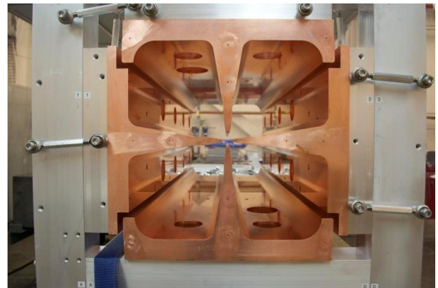
Figure 5: RFQ module in assembly fixture.
