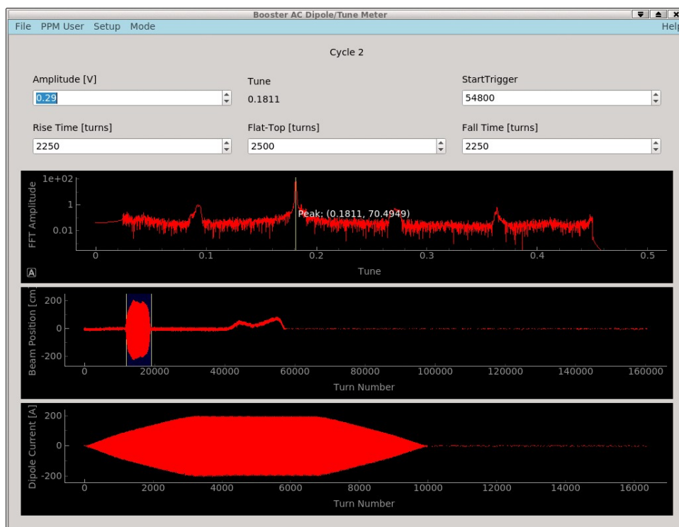
Figure 3.10: The Booster AC dipole application with ADO controls on top and 3 graphics panes of: FFT of vertical BPM data (top); vertical BPM data (middle); AC dipole current (bottom).
