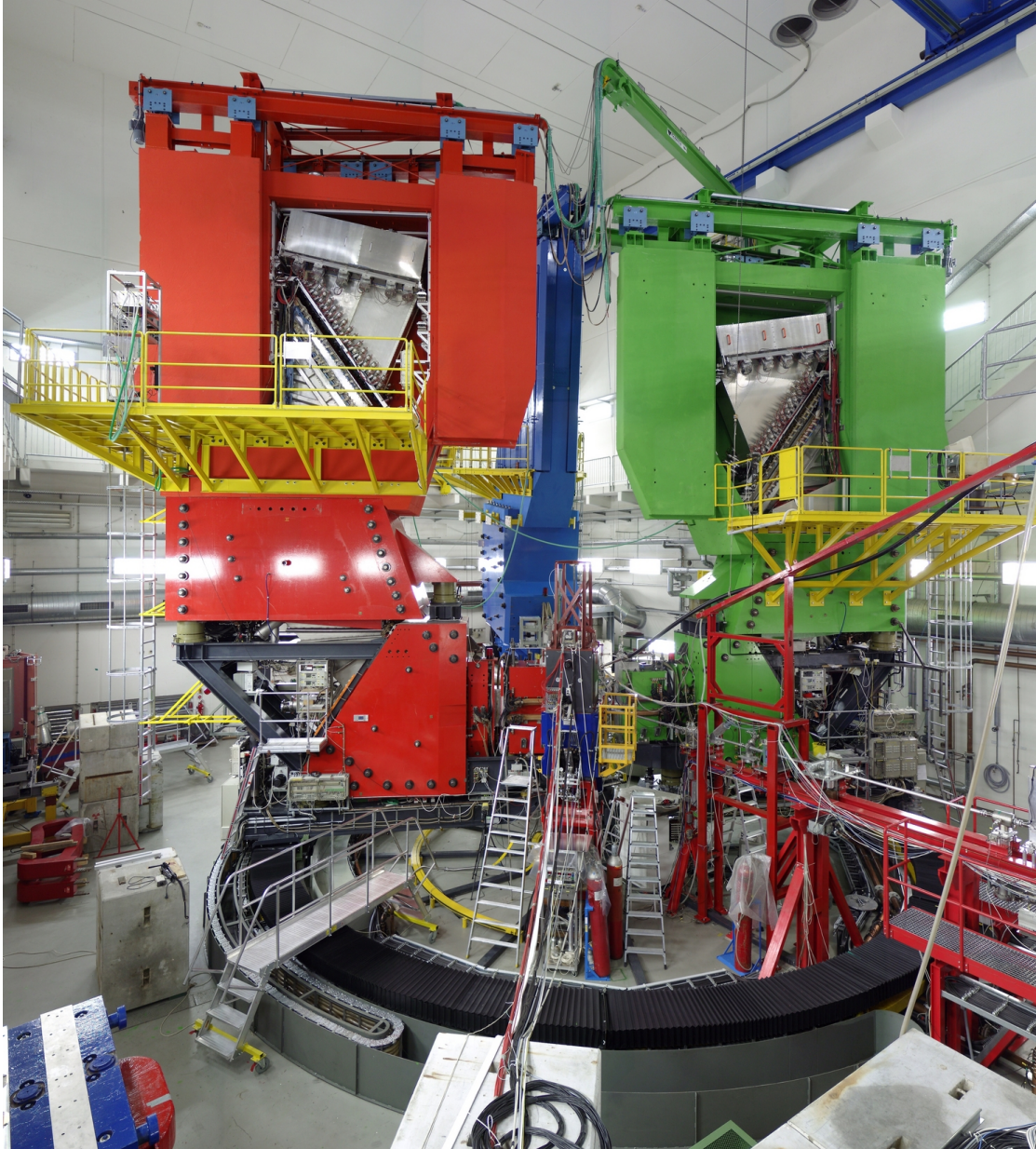
Figure 19: Picture of the A1 hall where the experiment was performed. The three spectrometers A (red), B (blue) and C (green) are visible. The shielding houses of Spec. A and Spec. C are opened and the detectors are visible. (source: [27])
