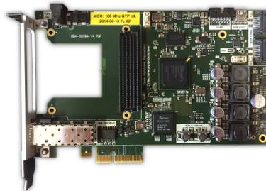
Figure 3: Simple PCIe FMC carrier (SPEC).
