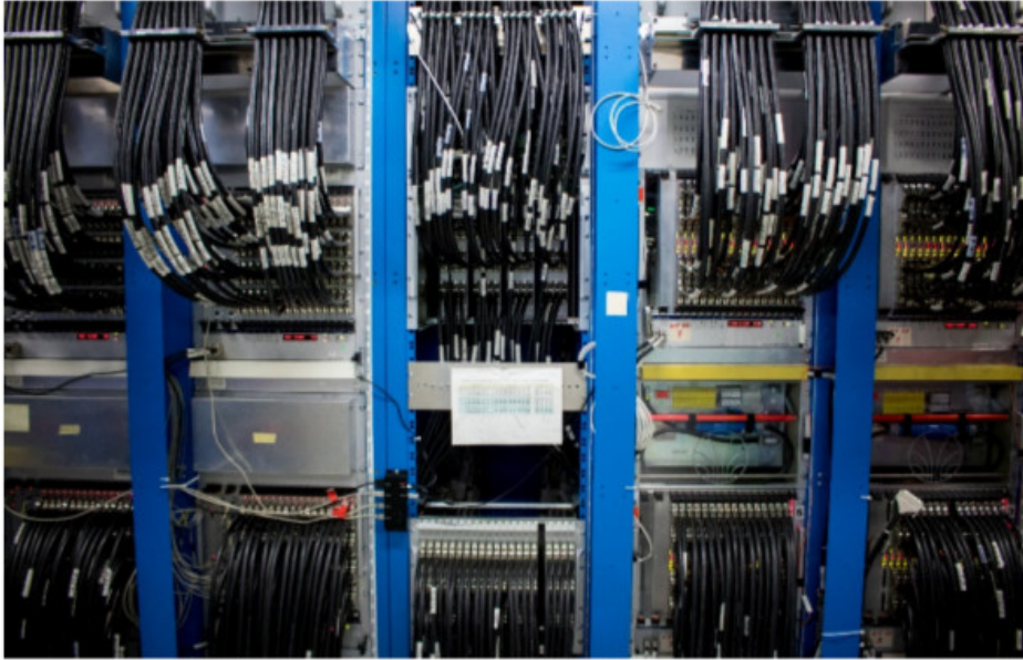
Figure 2.13: Racks of the first-level calorimeter trigger system installed close to the detector.
