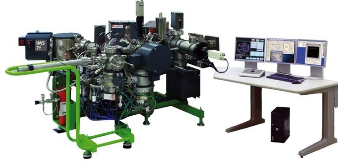
Figure 6.4: The CAMECA IMF 7F System where SIMS measurements were performed at GEMAC laboratory at the university Saint-Quentin-en-Yvelines at Versailles [102].
