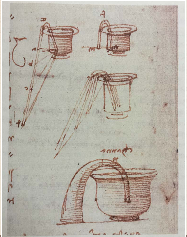
Fig. 12 One of the many drawings by Leonardo describing the functioning of the siphon. Leicester Codex, 3A, folio 34 verso.
