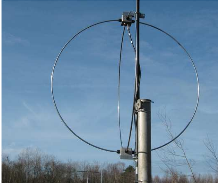
Figure 11.1: The Salla antenna during test measurements at the Nançay Radio Observatory. The Salla realizes a Beverage antenna as a dipole loop of 120 cm diameter. The antenna is readout at the top with an LNA. The amplified signal is guided through the antenna structure to the bottom.
