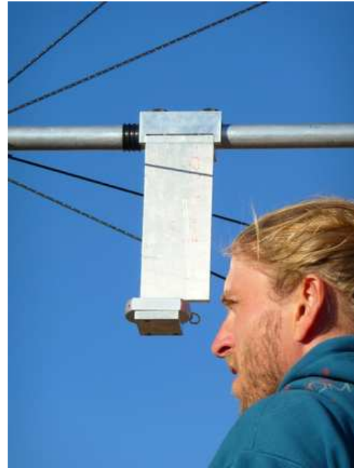
Figure 7.9: The compass is mounted on a bracket, especially designed to allow a torsion free fastening parallel to the lowest antenna dipole.
