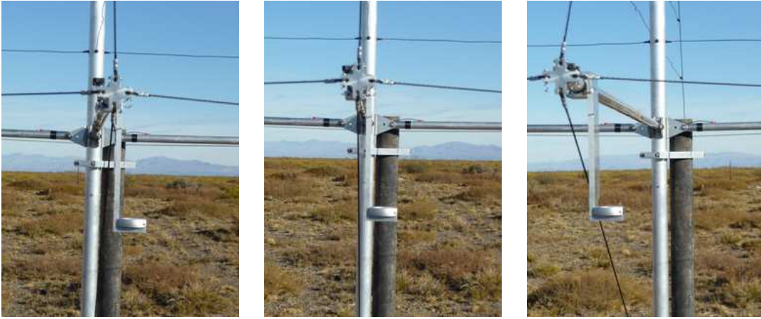
Figure 7.10: The compass mounting bracket is attached on the same side of the antenna as the metallic pole the antenna is attached to. In this way the influence of a possible magnetism of the pole is minimized as far as the pointing to the geo-magnetic North direction is concerned.
