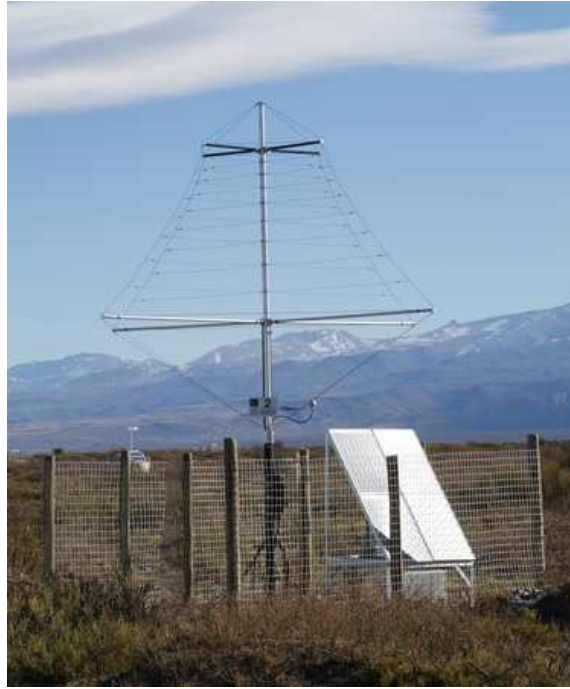
Figure 5.6: A radio-detector station installed at the AERA site. Visible is the 'Small Black Spider' LPDA, the GPS antenna and the solar panels above the electronics box.
