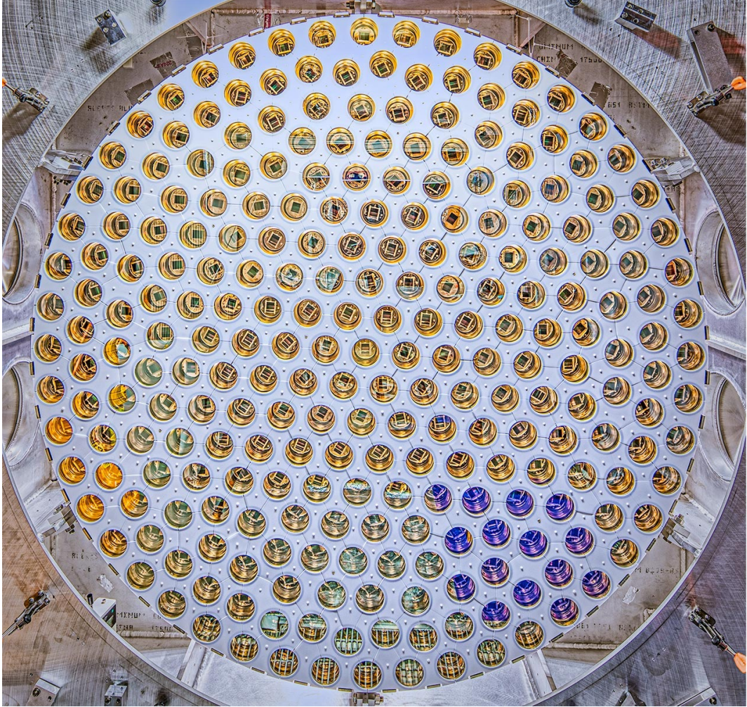
Figure 5.9: Image showing the top array PMT layout in LZ. The Top array employs a circular structure of PMT layout, with the outer ring of PMTs placed further than the TPC walls. This is to improve position reconstruction and light collection for events nearer to the walls of the TPC. In total, there are 253 PMTs in the Top array.
