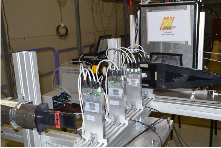
Figure 4.8: A closeup view of the telescope in the beam-test. Three of the telescope planes in aluminum enclosures are positioned on the beam path (from left to right). There is one trigger scintillator counter in front of the telescope and one behind the third telescope plane.
