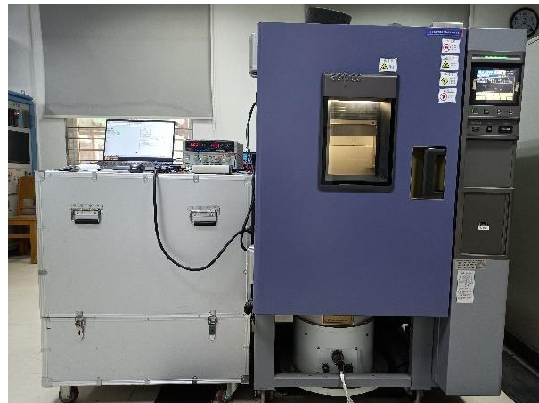
Figure 7. Scene of accelerometer temperature experiment.
