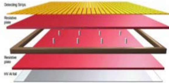
Figure 3.21. Resistive plate chamber layers ( http://cms.web.cern.ch/news/resistive-plate-chambers ).
