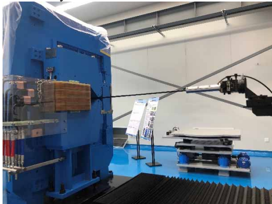
Figure 6: Superbend magnet being measured by a Hall probe measurement system.
