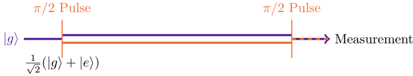
Figure 5.3: Internal-state atom interferometer: Atoms remain in the same spatial path but transition between internal states using coherent pulses. The phase difference accumulates due to energy differences between states.
