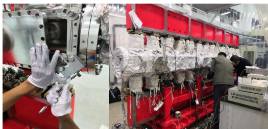
Figure 8: On the left, the side flange was being installed. On the right, final inspection before baking.
