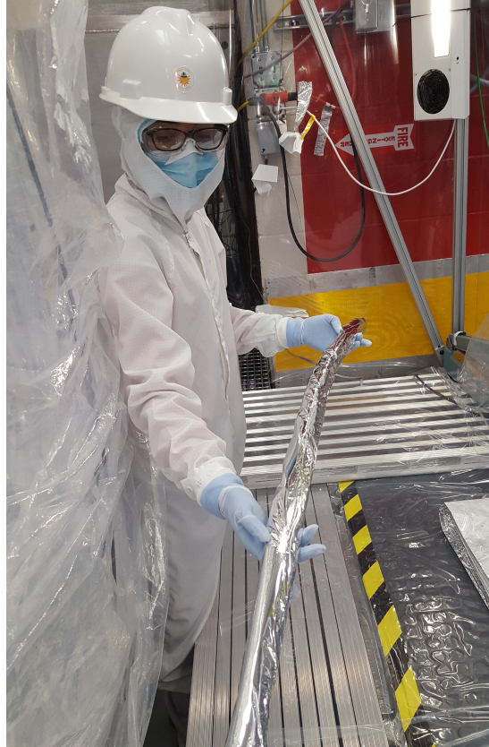
Figure 3.9 This author preparing an MLI wrapped thermosyphon line for installation on the ICV.
