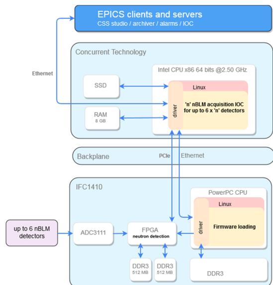
Figure 9: Data processing architecture for ESS nBLM.
