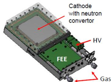
Figure 1: Detector schematic with its FEE.
