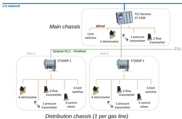
Figure 7: Gas chassis architecture. A PLC Siemens S7-1500 is inside the main gas chassis. Each distribution chassis has a Siemens ET200SP remote I/O module [8].
