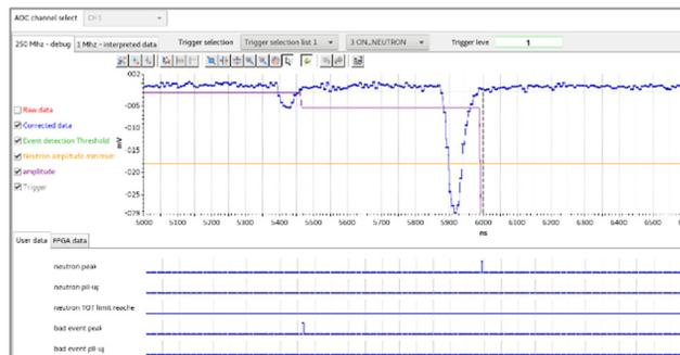
Figure 12: CS-Studio view of an event shape acquired with the scope functionality with an event configuration.
