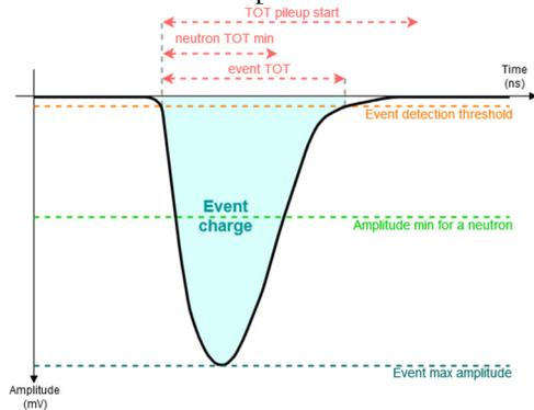
Figure 2: Typical event shape expected in a Micromegas detector.
