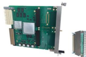
Figure 8: IOxOS boards: AMC board and FMC ADC module to the right [11].
