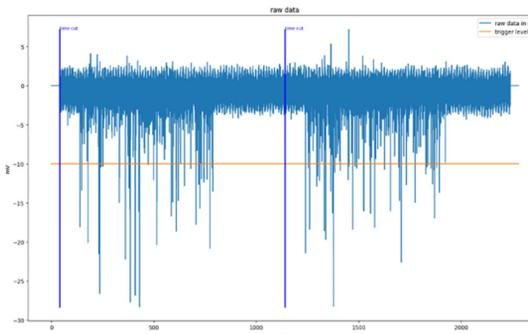
Figure 11: Display of interesting sections of the beam. With a trigger level a Python script concatenates and displays beam pulse data (trigger level, pre-trigger and post-trigger are set in the script).
