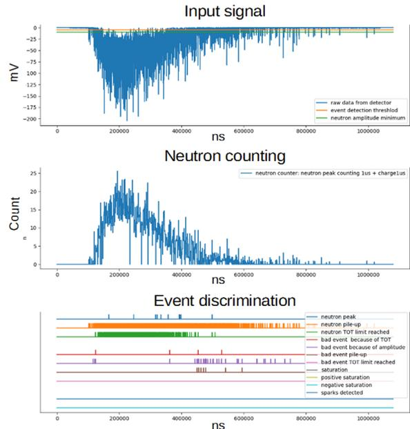
Figure 5: First graph is the IPHI experimental raw data and the second graph shows the results of events counting for a given configuration.
